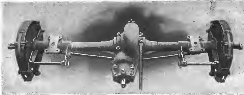
Rear Axle, Showing Means for Keeping Brakes from Dragging.
